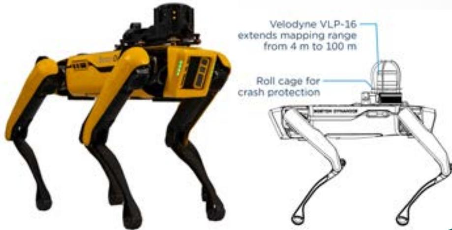
Dialog's Robotics division can provide the World-Leading Boston Dynamics legged and wheeled robots for Australian organisations use cases. Specialising in the Spot 4-legged robot solutions.
